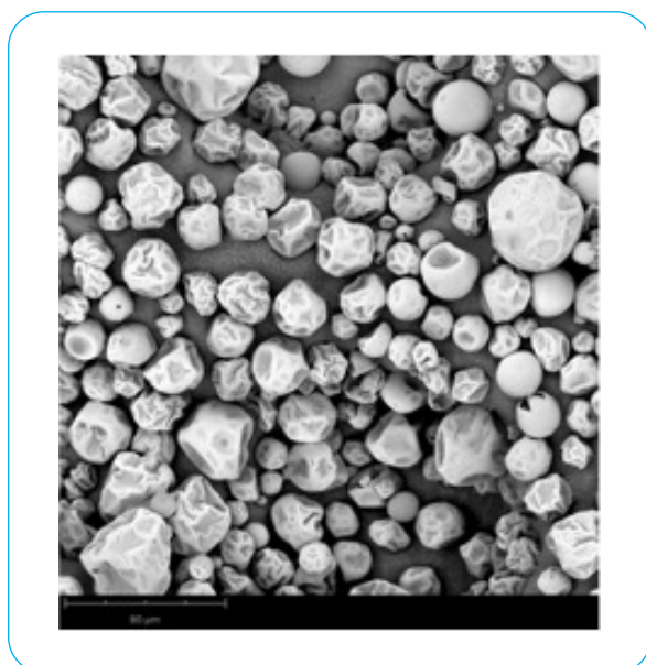
Image of Liposovit-Fe® liposome structures using x1000 magnification under scanning electron microscope.
