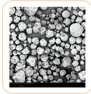
Image of Lipsovit® liposome structures using x1000 magnification under scanning electron microscope.
